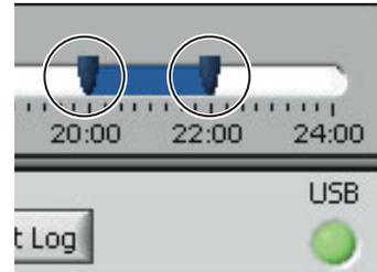
The arrows on each end of the slide bar (circled) designate the start and stop time of each cycle.
